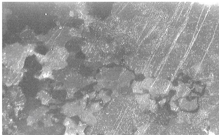
Fig. 5. Detrital grain of quartz, late katagenesis, crushing of grain into blocks and granules; purification of granules from fluids; side lighting; magnification 100 X
