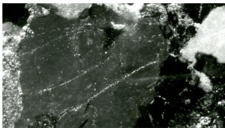
Fig. 1. Bem's stripes in detrital quartz grains, side illumination, thin section, magnification 100^{\times} , Donbass sandstone
